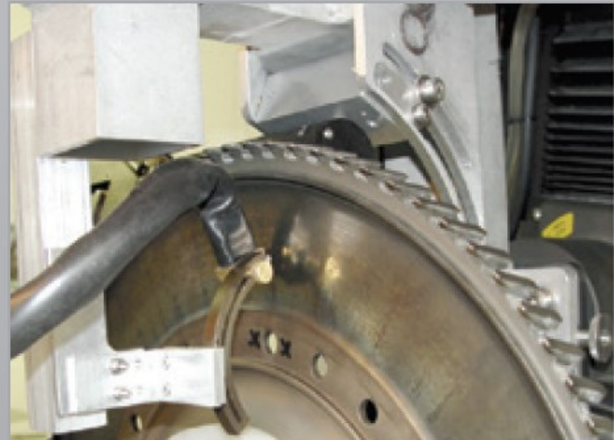
Measuring Residual Stress Inside a Bolthole
