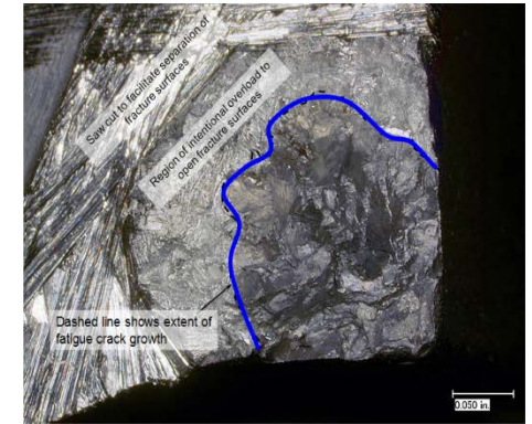
Observed crack shape for LSP (Frame 2 test article)
